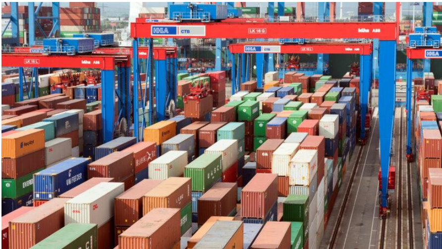
Gambar 4. 2 ASC - Automated Stacking Cranes [45].
